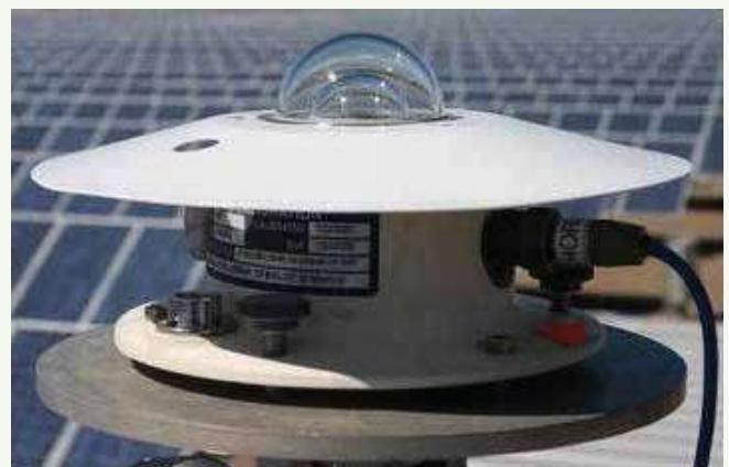
Figure 11: Pyranometer Measuring GHI Image
