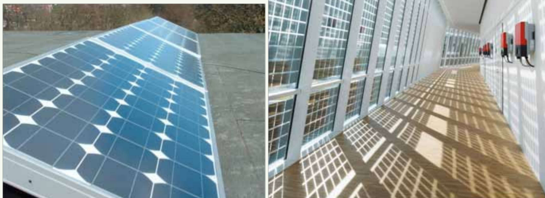
Figure 35: BAPV (Left) and BIPV (Right) Systems
